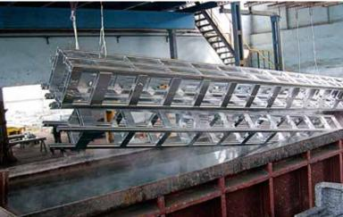
Hot dip galvanizing, as a method of contemporary corrosion protection, is a solution which fulfils all the requirements in terms of durability, good appearance and environmental care. Correctly performed zinc coating, depending on the exposure rating of working environment, guarantees full protection for as long as 50 years.
